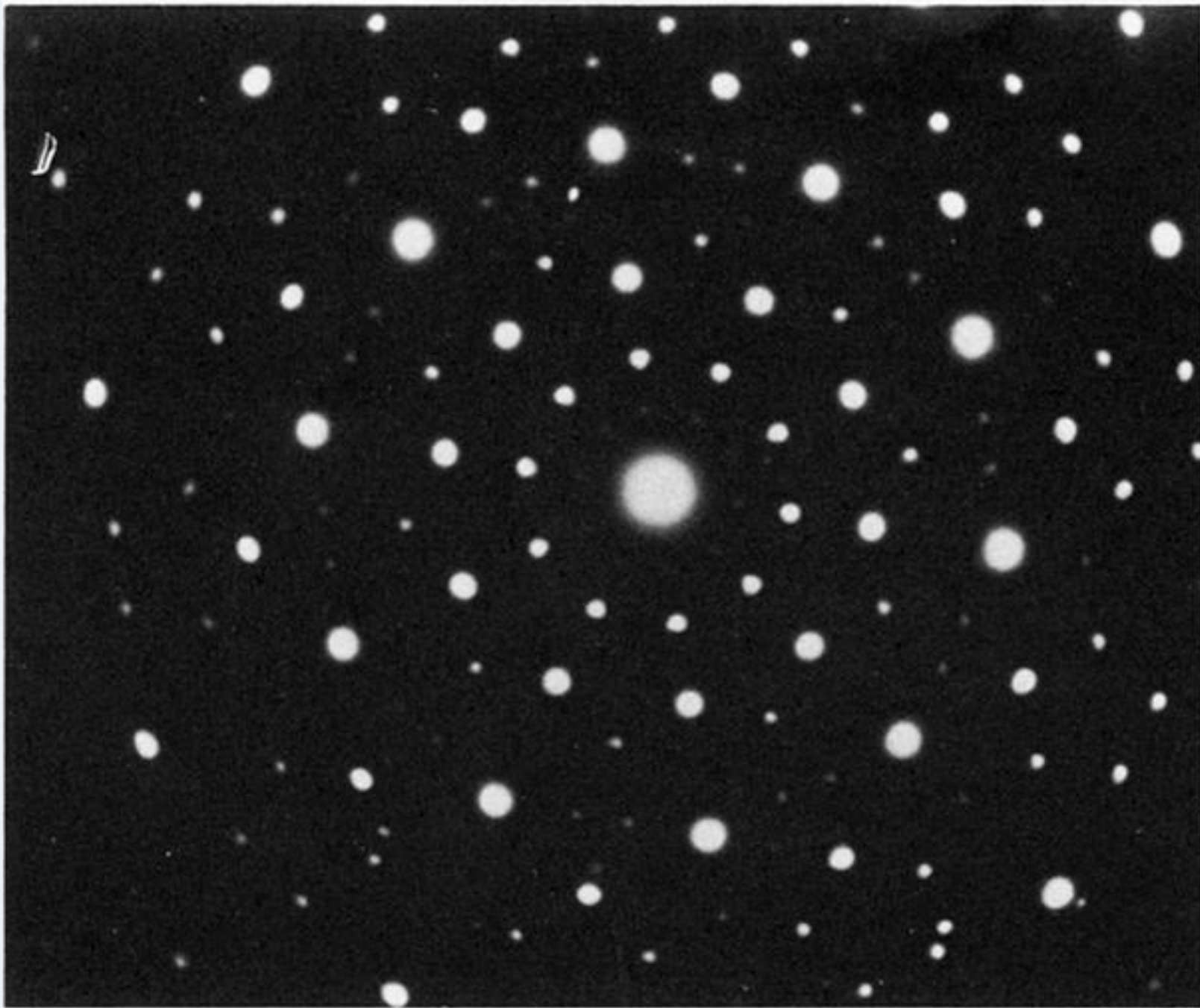
FIGURE 1. Diffraction pattern from melt-spun Al-15% Mn.
